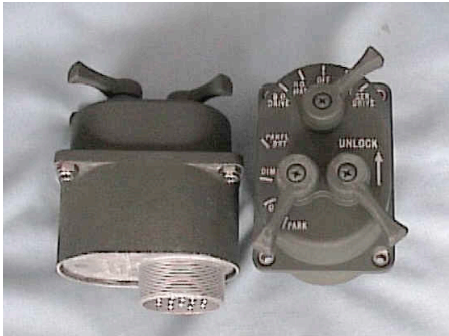
M-Series 3-lever light switch assembly, used on all M-series military vehicles.
