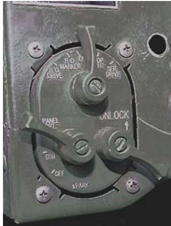
M-Series 3-lever light switch installed in HMMWV dash.
